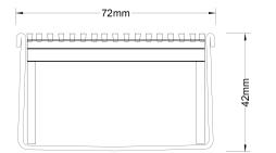
Grates longer than 1500mm supplied in sections. Tile Inserts longer than 1200mm supplied in sections. Channels over 3000mm supplied in sections with joiner. +/-2mm tolerance on dimensions.
